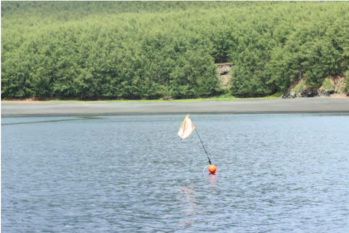
Figure 2-8. Moored Sonobuoy with Float and Flag for Retrieval
