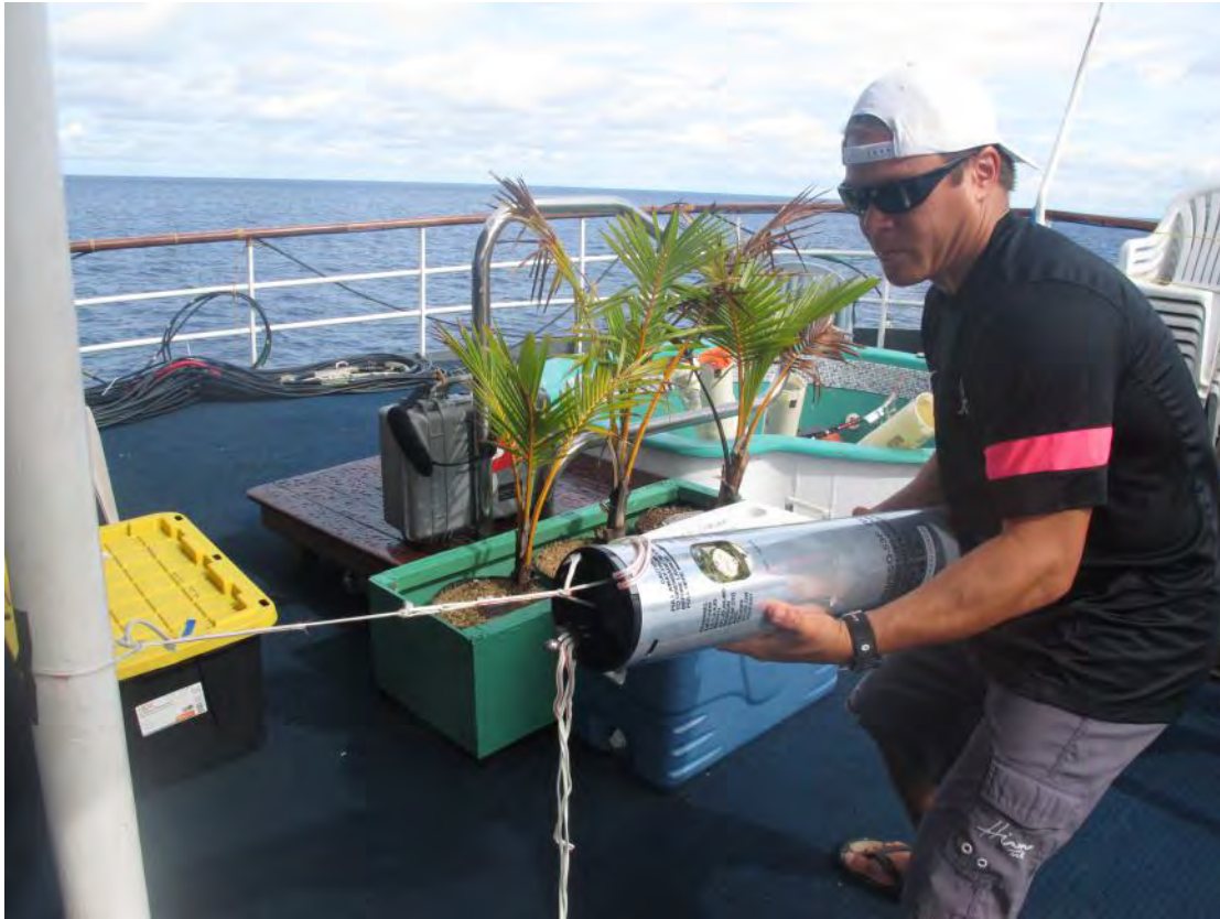
Removing the cap of the sonobuoys in preparation for nighttime deployment at the moored sites
