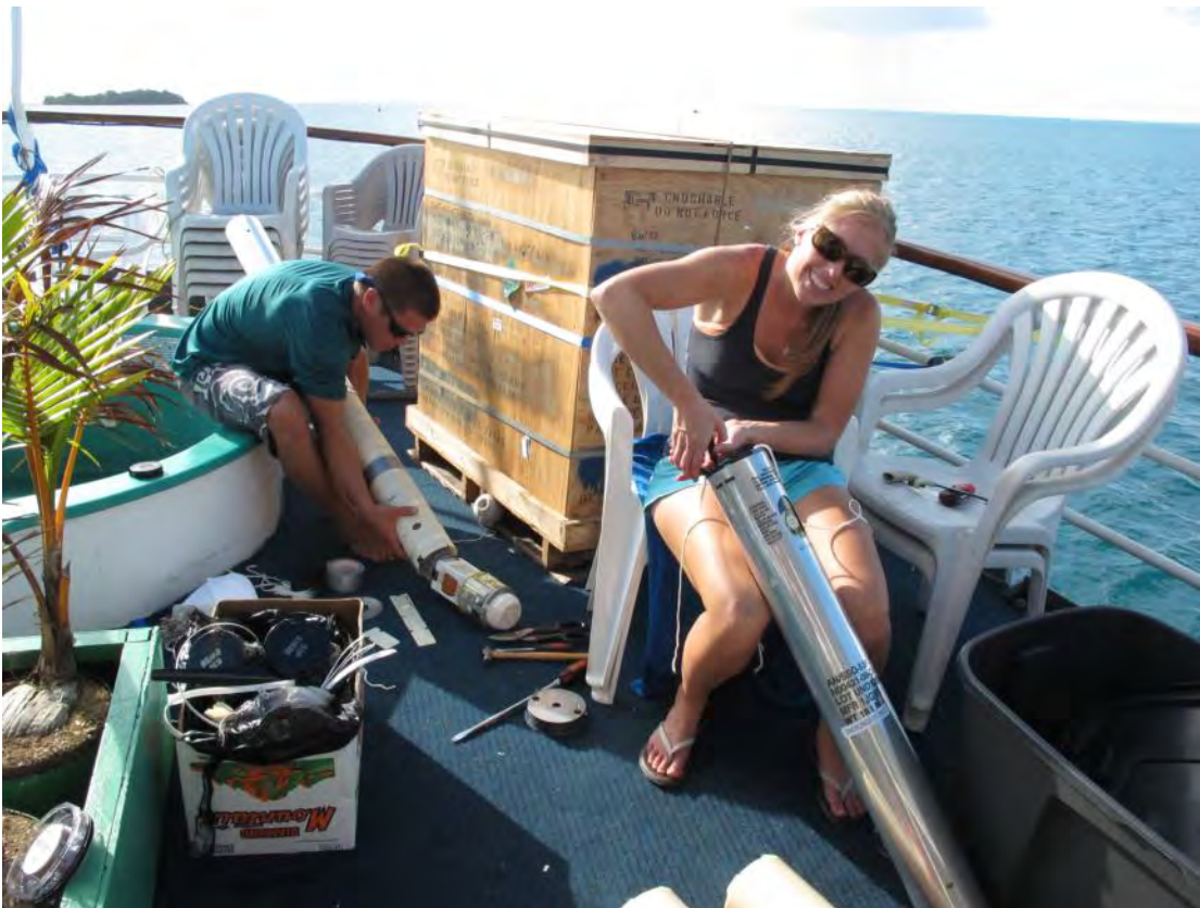
Preparing the sonobuoy assembly for nighttime deployment at the moored sites
