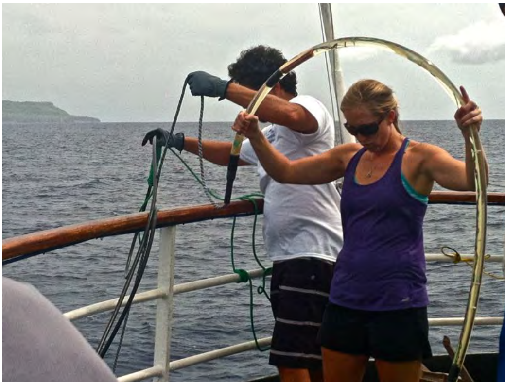
Figure 2-7. Deployment of the Towed Array from the Aft Deck of the Thorfinn
