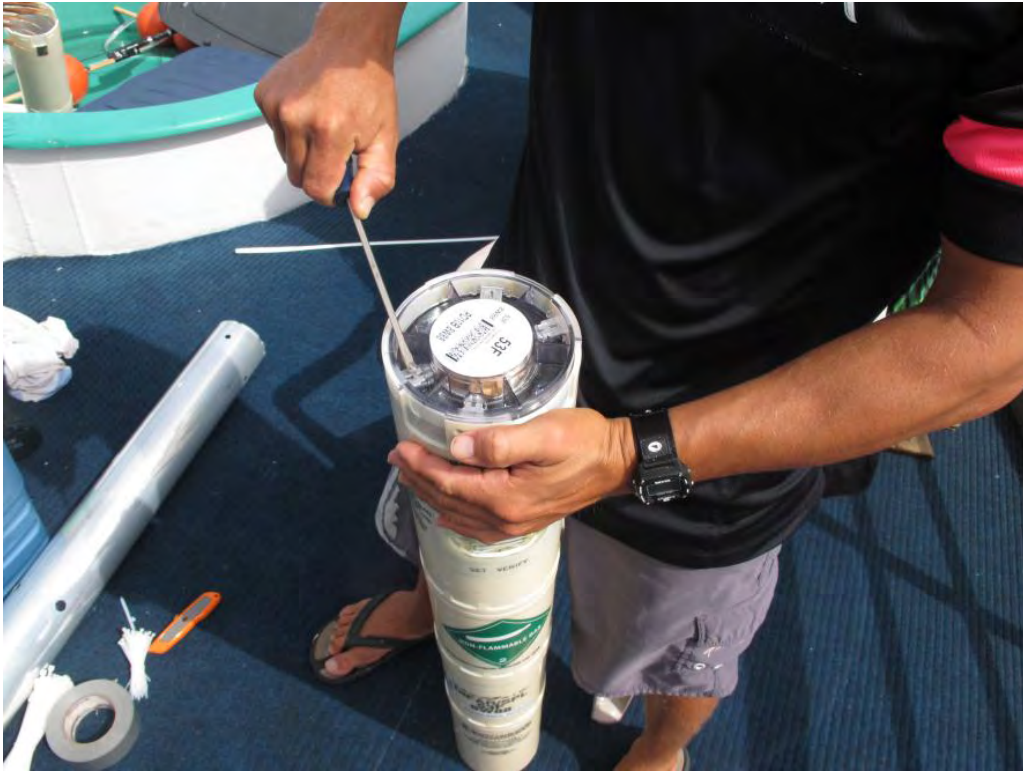
Preparing for lid removal of the sonobuoys for nighttime deployment at the moored sites
